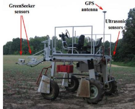
**Fig. 5:** Variable rate fertilizer applicator for cotton
