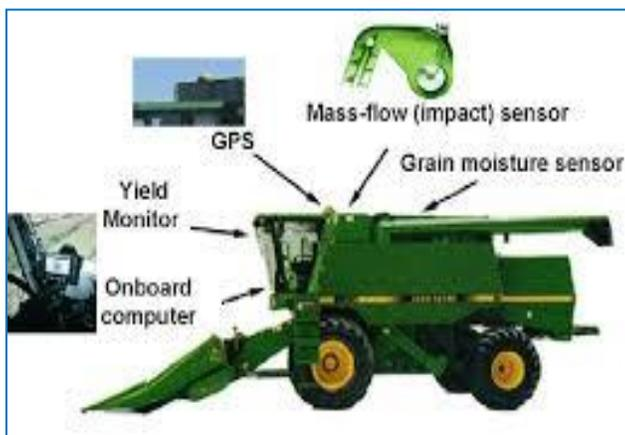
**Fig. 6:** Combine Harvester with yield monitor on board computer, GPS and sensors
